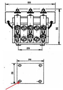
Mounting Hole dimension 4 mm dia of 4 Nos.
